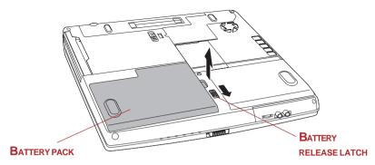
Figure 6-1 Releasing the battery pack
